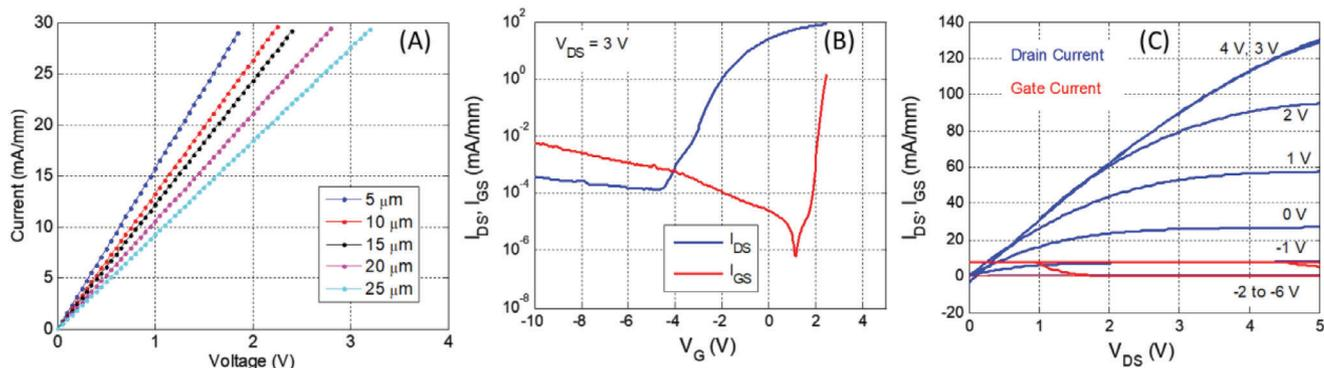
**Figure 2.** Electrical sweeps of PC85/50 for A) CTLM characterization, B) drain and gate current as a function of gate bias ( $V_{DS} = 3$  V), C) drain and gate current versus drain-to-source bias ( $V_{GS} = -6$ – $4$  V in 1 V increments).
