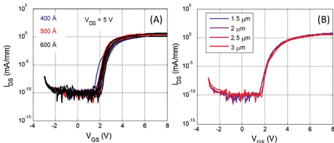
**Figure 4.**  $I/V$  sweeps for A) gate recess depths of 400, 500, and 600 Å and B) variable gate length of 1.5, 2, 2.5, and 3  $\mu\text{m}$ . ( $V_{DS} = 5$  V).
