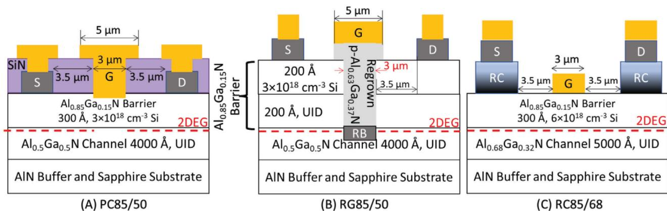
**Figure 1.** Transistor epitaxial architectures and layout indicating locations of the source (S), gate (G), drain (D), regrown barrier (RB), regrown contact (RC), and 2D electron gas (2DEG).
