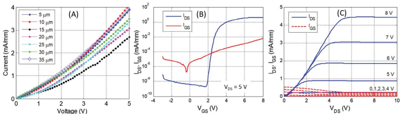
**Figure 3.** RG85/50 electrical sweeps. A) CTLM, B) drain current versus gate bias ( $V_{DS} = 5$  V), C) drain current versus drain-to-source ( $V_{GS} = 0$  to 8 V in 1 V increments).
