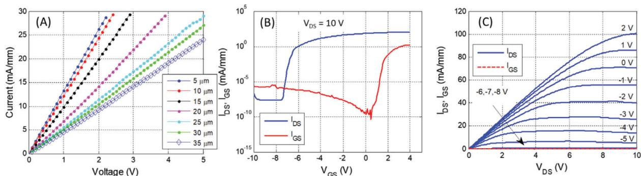
**Figure 5.** RC85/68 electrical sweeps. A) CTLM, B) drain current versus gate bias ( $V_{DS} = 10$  V), C) drain current versus drain-to-source bias ( $V_G = 2$ — $8$  in 1 V increments).
